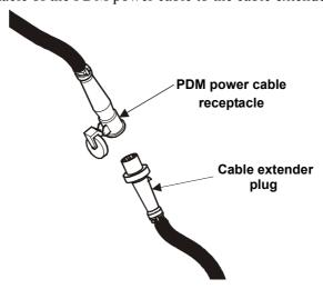
2 Run the receptacle end of the attached cable extender through a cable trough to the rack or enclosure with the equipment to which you wish to feed power.
